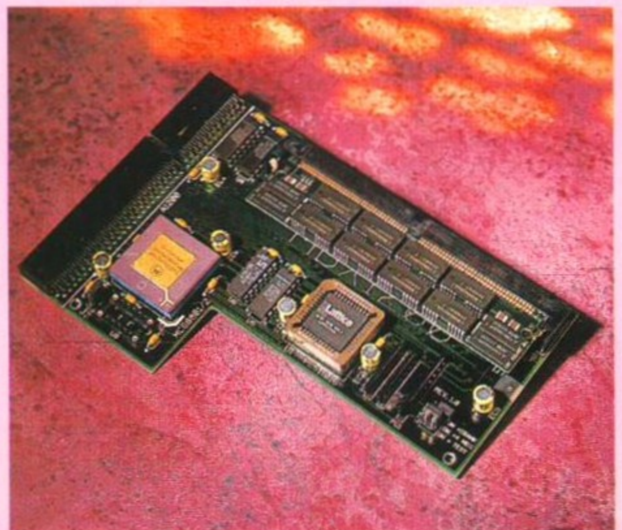
The MicroBotics MBX1200, showing off its 68881 co-processor, and the 4Mb SIMM fitted to the review model.
