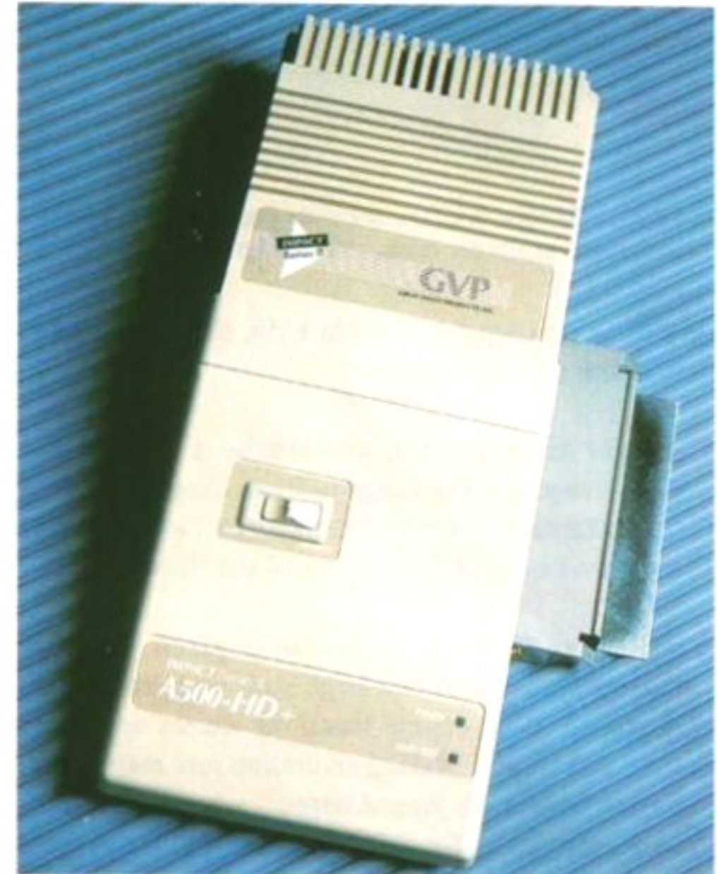
Hard drives, like this GVP, contain moving parts, and faults are often the result of loose connections.
